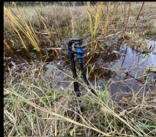
Solar-Powered Well-Point System with Automated Micro-Nebulisers to secure topsoil moisture for standing freshwater habitats
